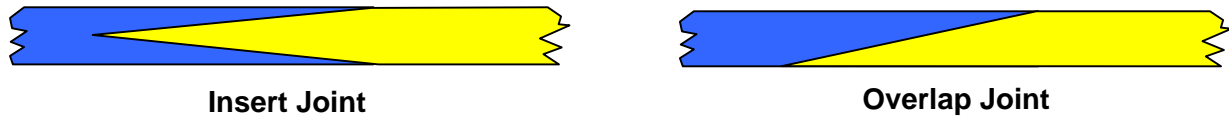
Figure 6. Transition of carbon fiber composite to glass fiber composite in molded parts.
