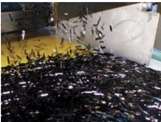
Chopped carbon fiber falls onto a Lytex resin during the manufacture of Lytex 4149 Engineered Structural Composite molding compound.
